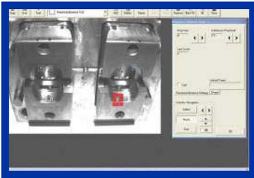
Setting up for a new mold or running an existing setup is very straight-forward. A new mold setup can be implemented in just minutes and if a change is made to an existing job, the "Teach" function captures and updates the reference image with the touch of a button. Once a setup has been completed, it can be saved to a disk and the job can be run by executing a single "Teach" cycle.
